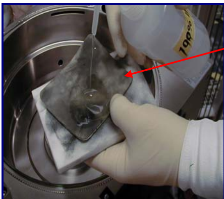
Fig 2: Lightly dampen 800 Grit ScrubPAD w/IPA
