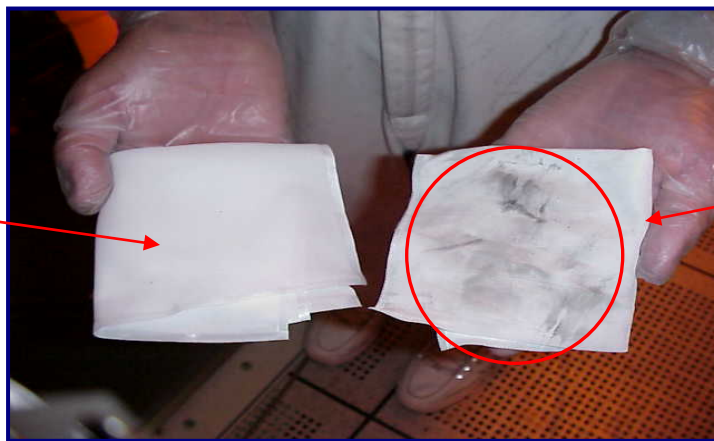
Fig 6a: Current fab wiper after completely wiping the AMAT HDP Chamber
