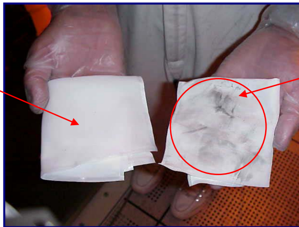
Fig 15a: Current fab wiper after completely wiping HDP dome
