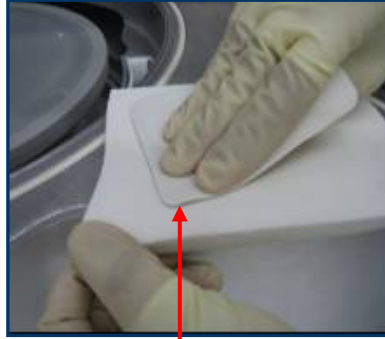
Fig 10: Pull ScrubPAD across UltraSOLV ® Sponge
