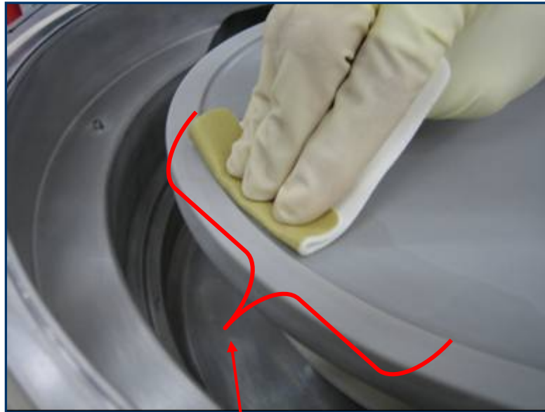
Fig 7: Fold Diamond ScrubPAD over and scrub a small area
