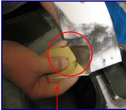
Fig 5: ScrubPAD loaded with deposition
