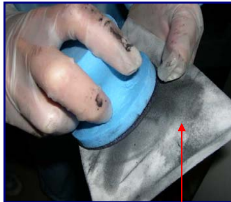
Fig 2: Pull & twist ScrubDISK ® across UltraSOLV ® Sponge
