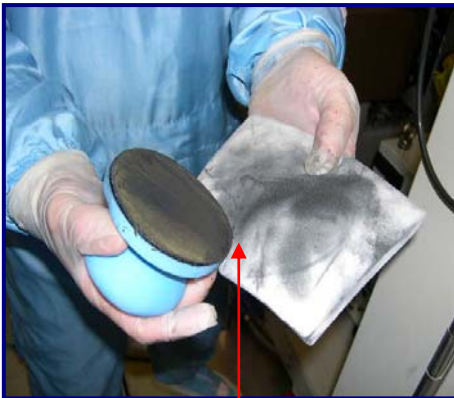
Fig 1: ScrubDISK ® loaded with deposition
