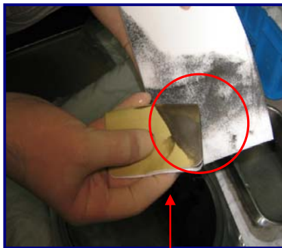
Fig 2: ScrubPAD loaded with deposition
