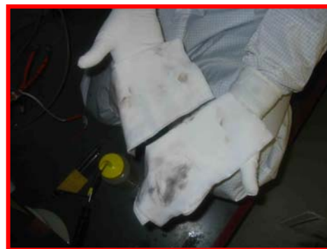
Foamex HT5790S MiraWIPE ® results after wiping exact same area as before.
