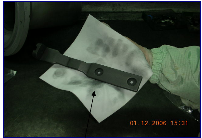
GRAPHITE PIECE WIPED WITH ULTRASOLV® FOAM WIPER AFTER BEING WIPED WITH STANDARD FAB WIPER ○ MUCH MORE PARTICLES REMOVED WITH ULTRASOLV® FOAM WIPE
