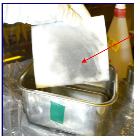
Fig 1: UltraSOLV® Sponge loaded with deposition
