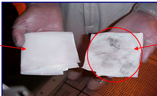
Fig 22b: Particles picked up using HT5790S MiraWIPES ® after completely wiping with current fab wiper
