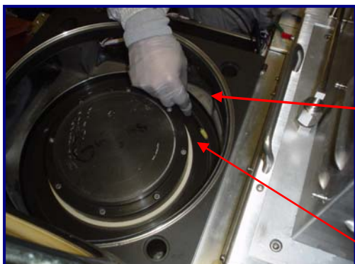
280 Grit Diamond ScrubTIP ® cleaning track on bottom of Chamber
