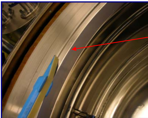
Fig 23 & 24: ScrubWRIGHT® PEN scrubbing along the chamber flange
