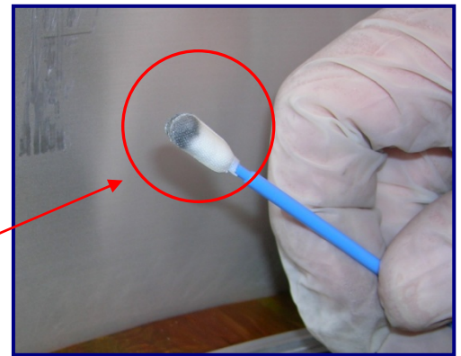
Fig 13 & 14: What the HT1511FC MiraSWAB® was able to effectively remove from upper chamber ring
