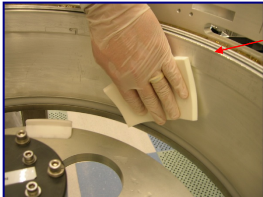
Fig 7: Deposition on UltraSOLV ® Sponge
