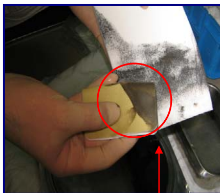
Fig 8: ScrubPAD loaded with deposition
