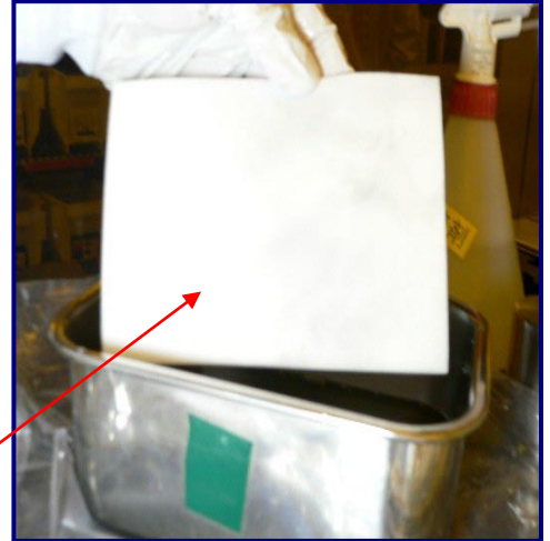
Fig 4: UltraSOLV ® Sponge loaded with deposition
