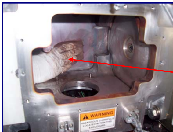
Fig 2: Scrub small area using 280 Grit Diamond ScrubPAD
