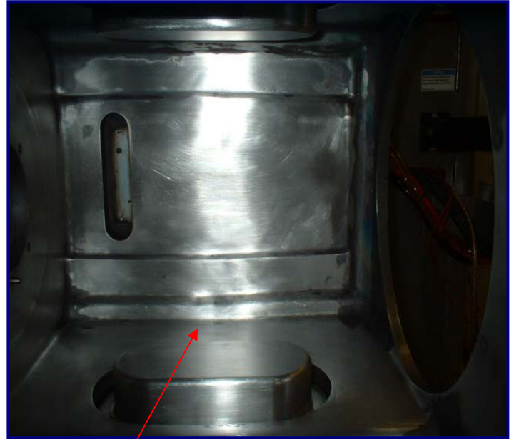
Fig 10 & 11: PM completed using only DI water and IPA for final wipe-down
