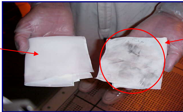
Fig 6b: Particles picked up using HT5790S MiraWIPES® after completely wiping with current fab wiper
