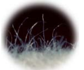
Standard Polyester Wiper After Use on Bead Blasted Tool Surface
