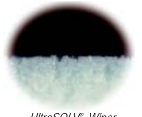
UltraSOLV® Wiper After Use on Bead Blasted Tool Surface
