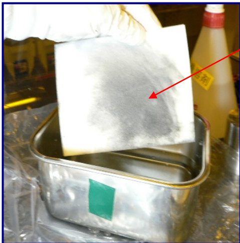
Fig 9: UltraSOLV ® Sponge loaded with deposition
