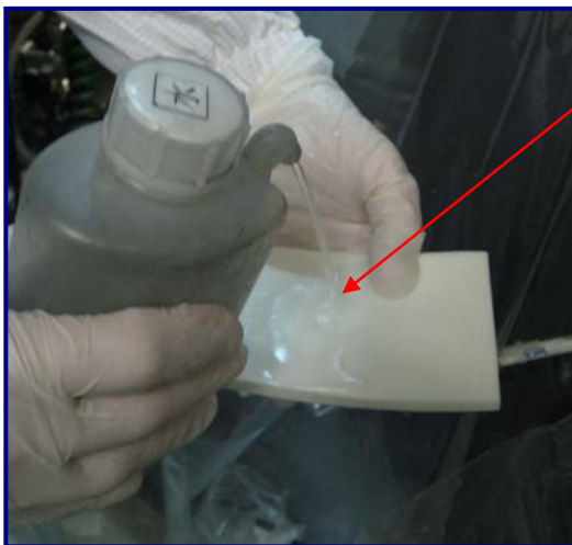
Fig 2: Dampen UltraSOLV ® Sponge with DI water
