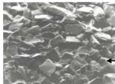
SiC abrasive crystals for more complete probe tip cleaning.
