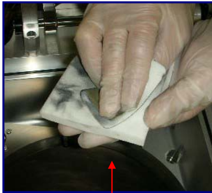
Fig 6: Pull ScrubPAD across UltraSOLV ® Sponge
