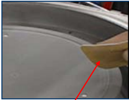
Fig 9: ScrubPAD loaded with deposition
