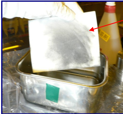
Fig 4: Loaded-up UltraSOLV ® Sponge
