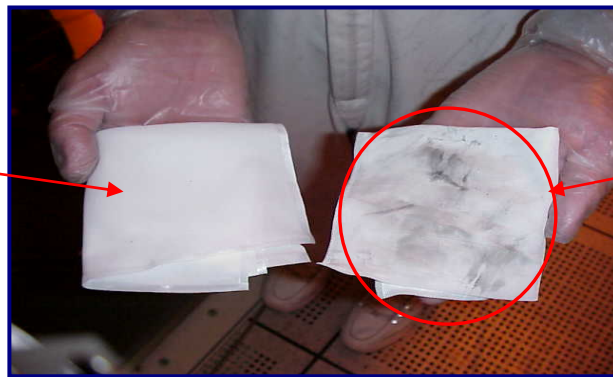
Fig 8b: Particles picked up using HT5790S MiraWIPES® after completely wiping with current fab wiper
