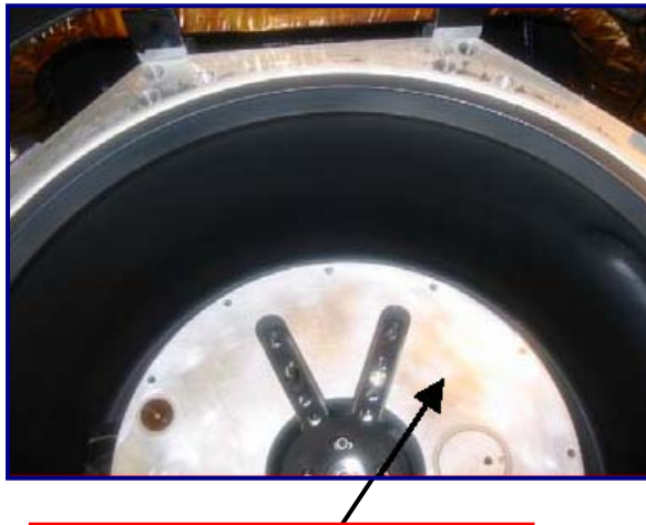
Fig 10: Cleaned cathode area
