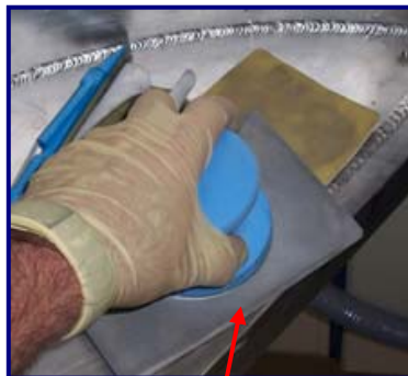
Fig 8: Pull ScrubPAD across UltraSOLV ® Sponge
