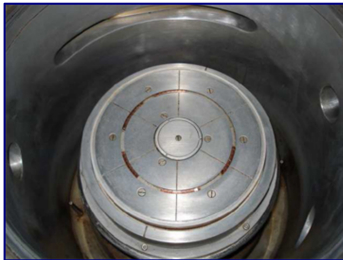
FIG 10: COMPLETED STS-RIE CHAMBER WALL ASSEMBLY SCRUB
