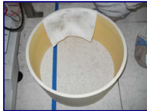
Fig 14 & 15: Use UltraSOLV ® foam wiper dampened with IPA to clean the ceramic and bead blasted parts
