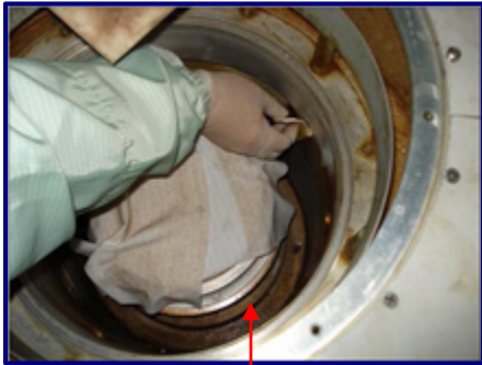
Fig 3: 360 Grit Diamond ScrubPad scrubbing entire chamber and chamber wall
