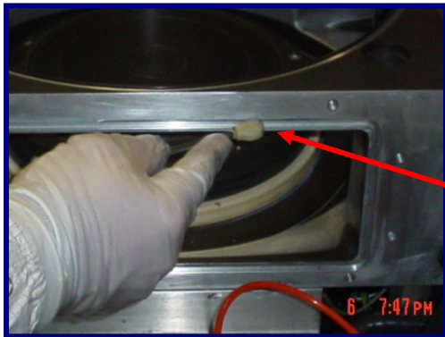
Fig 7 & 8: Using Diamond ScrubTIP ® to clean hard to reach areas and o-ring grooves
