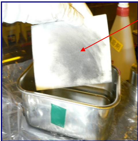
Fig 5: UltraSOLV ® Sponge loaded with deposition
