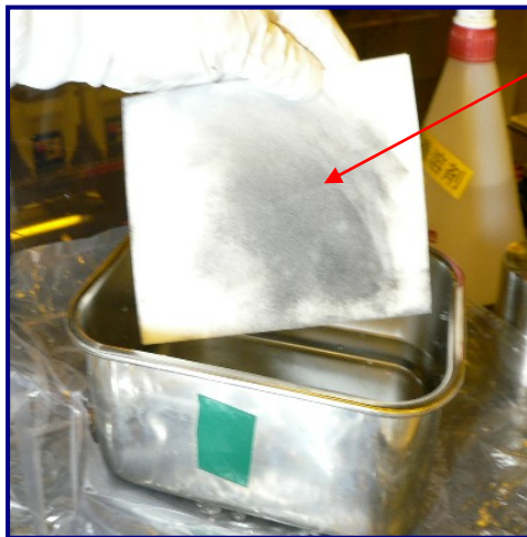
Fig 4: UltraSOLV® Sponge loaded with deposition
