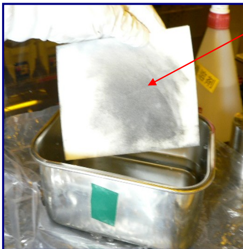
Fig 5: UltraSOLV ® Sponge loaded with deposition
