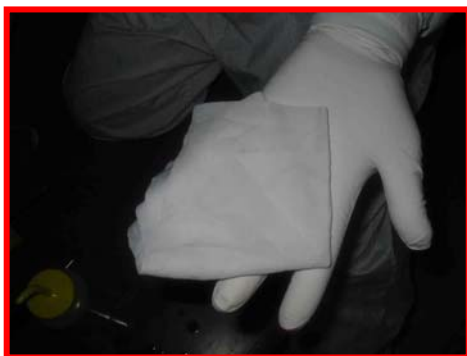
Standard fab wiper after completing Final Wipe of Chamber.
