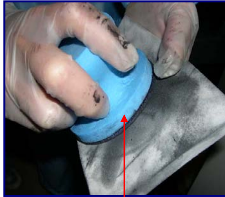
Fig 6: Pull & twist ScrubDISK ® across UltraSOLV ® Sponge
