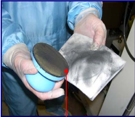
Fig 5: ScrubDISK ® loaded with deposition
