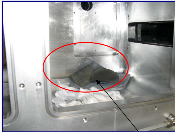
HAZARDOUS WASTE ACCUMULATED
