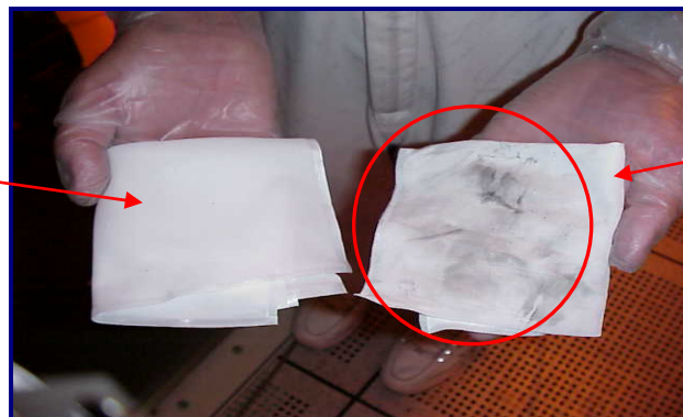
Fig 10a: Current fab wiper after completely wiping Varian VIISTA
