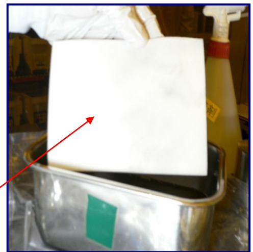
Fig 3: UltraSOLV ® Sponge loaded with deposition
