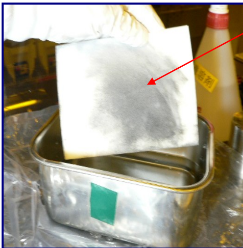
Fig 3: UltraSOLV ® Sponge loaded with deposition
