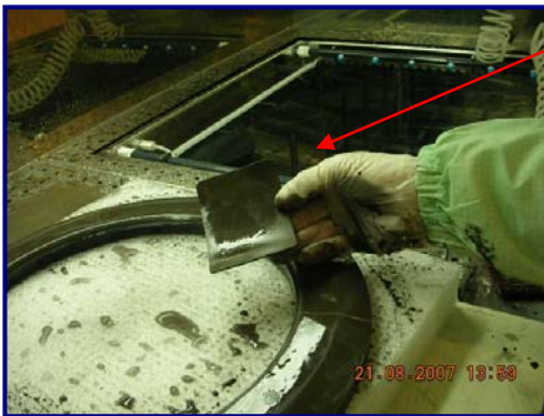
Fig 5: ScrubPAD loaded up with deposition
