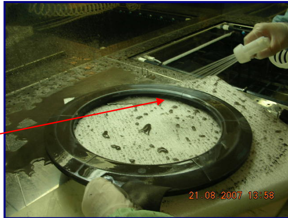
Fig 4: Rinsing off the electrode with DI water
