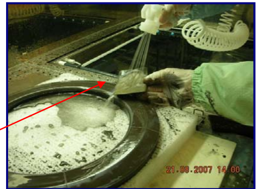
Fig 5: ScrubPAD loaded up with deposition
