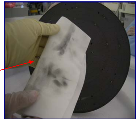
Fig 11: Particles removed by UltraSOLV® Foam Wiper AFTER soaking in Ultrasonic Sink
