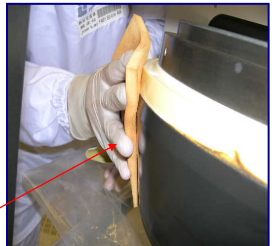
Fig 12: UltraSOLV ® Sponge removing scrubbed deposition from e-chuck
