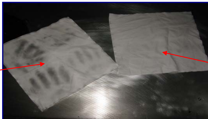
Fig 14a: What the MiraWIPE ® was able to remove, AFTER the standard fab wiper
