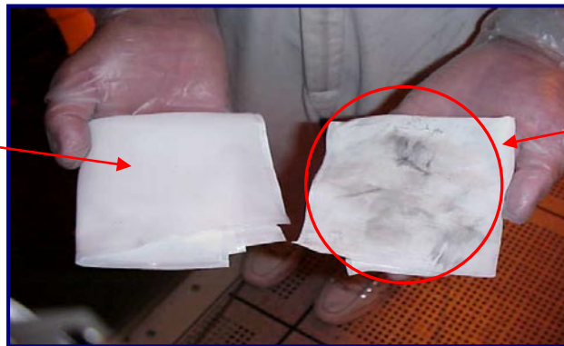
Fig 9b: Particles picked up using HT5790S MiraWIPES® after completely wiping with current fab wiper
