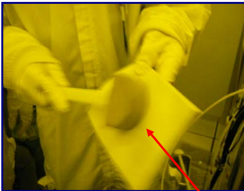
Fig 14 & 15: Unloading Diamond ScrubPAD onto UltraSOLV ® Sponge
