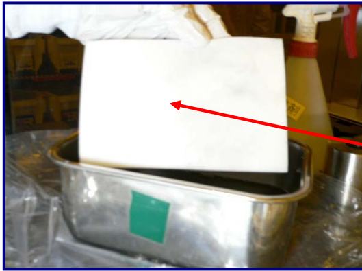
Fig 13: Dampen HT4754 UltraSOLV ® Sponge in DI water
