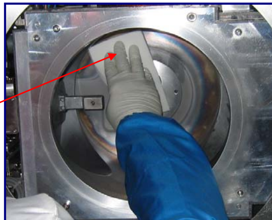
Fig 2: Foamtec International UltraSOLV ® Sponge pre-wiping GSD Source
