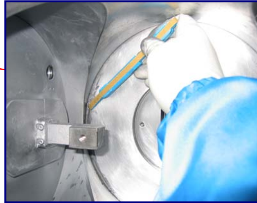
Fig 17: ScrubWRIGHT™ Pen scrubbing corners in source chamber
