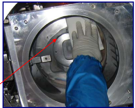
Fig 5: Dampened UltraSOLV ® Sponge preparing to wipe chamber
