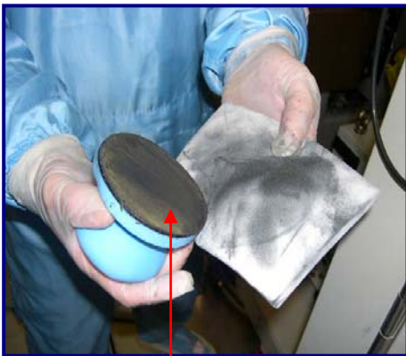
Fig 2: ScrubDISK ® loaded with deposition
