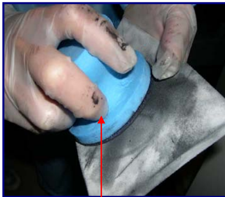
Fig 3: Pull & twist ScrubDISK ® across UltraSOLV ® Sponge
