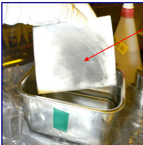
Fig 6: UltraSOLV ® Sponge free of deposition after rinse in DI water
