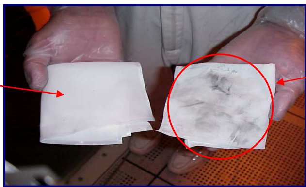
Fig 13a: Current fab wiper after completely wiping Novellus Concept 2
