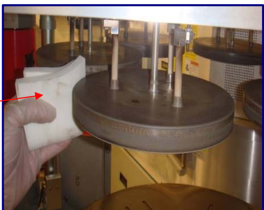
Fig 14 & 15: UltraSOLV® Sponge wiping top portion of Concept 2 Chamber
