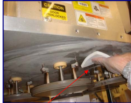
Fig 16 & 17: Scrubbing top of Concept 2 Chamber using same scrubbing technique described above on Chamber Wall Clean
