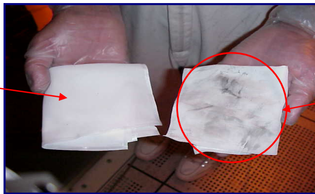
Fig 30b: Particles picked up using HT5790S MiraWIPES ® after completely wiping with current fab wiper
