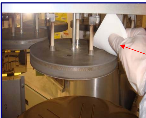
Fig 14 & 15: UltraSOLV® Sponge wiping top portion of Concept 2 Chamber
