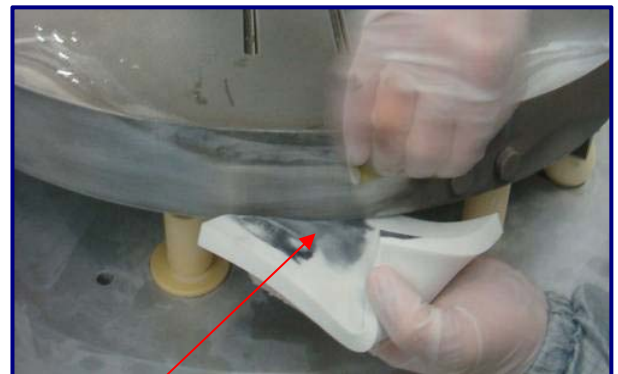
Fig 24 & 25: 180 Grit Diamond ScrubPAD w/UltraSOLV ® Sponge cleaning the side of heater block
