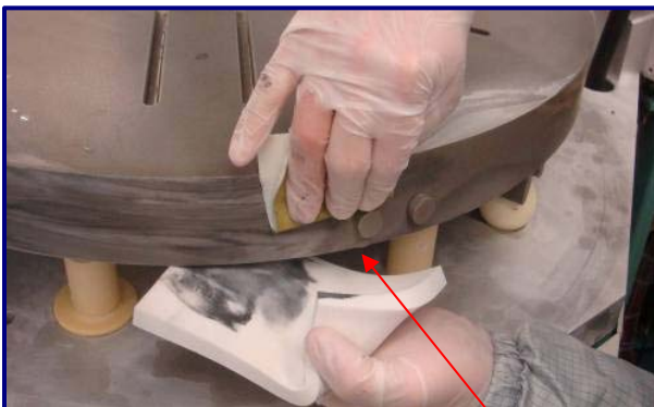
Fig 24 & 25: 180 Grit Diamond ScrubPAD w/UltraSOLV ® Sponge cleaning the side of heater block
