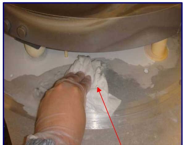
Fig 29: Wiping area below heater block with DI water saturated MiraWIPE ®
