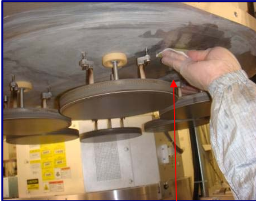
Fig 16 & 17: Scrubbing top of Concept 2 Chamber using same scrubbing technique described above on Chamber Wall Clean
