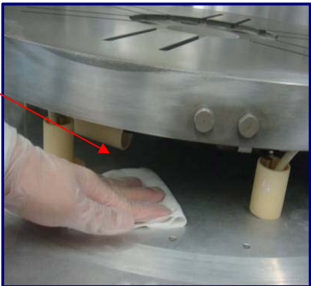
Fig 31 & 32: IPA saturated MiraWIPE ® wiping all areas of heater block and beneath heater block
