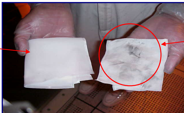
Fig 14a: Current fab wiper after completely wiping process chamber
