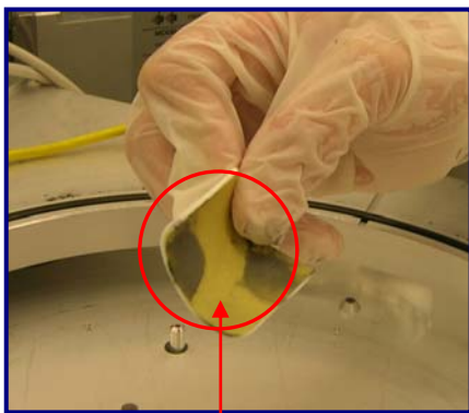
Fig 5: ScrubPAD loaded with deposition
