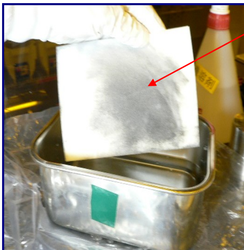
Fig 8: UltraSOLV® Sponge loaded with deposition
