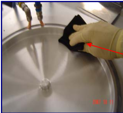
Fig 3: Visible airborne particles accumulated from surrounding areas of Degas Chamber
