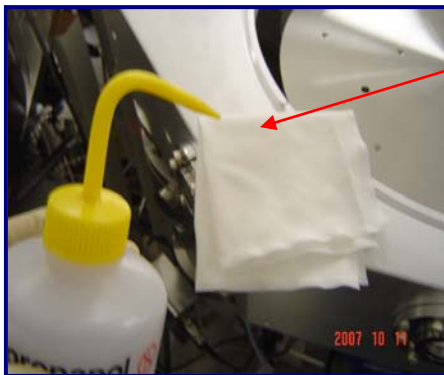
Fig 22: Dampen the HT5790S MiraWIPE ® with IPA
