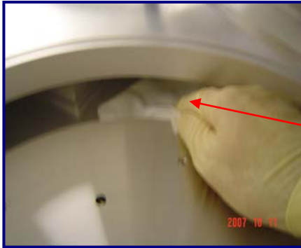
Fig 37, 38 & 39: Using MiraWIPES ® to wipe out all remaining areas of Degas Chamber
