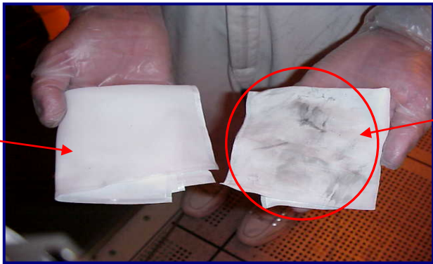
Fig 24b: Particles picked up using HT5790S MiraWIPES® after completely wiping with current fab wiper
