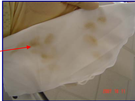
Fig 29: Deposition removed by HT5790S MiraWIPES ® on Degas Reflector
