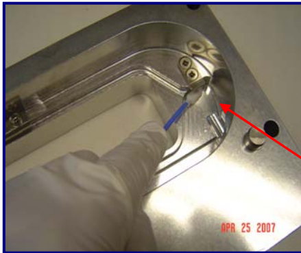
Fig 23 - 27: MiraSWAB® and MiraWIPE® effectively wiping cover of VAT valve sealing plate
