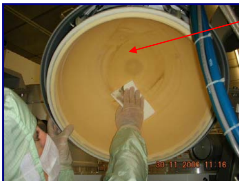
Fig 6: UltraSOLV ® Sponge wiping area free of deposition
