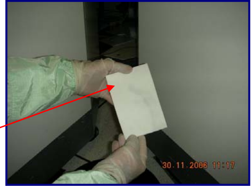
Fig 8: UltraSOLV® sponge loaded with deposition
