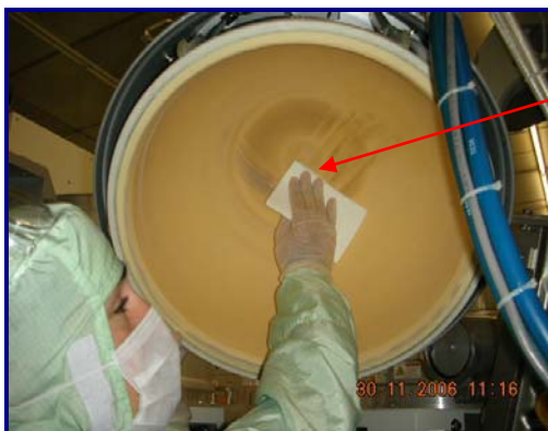
Fig 2: UltraSOLV ® Sponge performing initial wipe of ceramic dome
