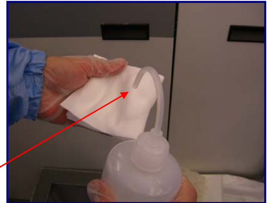
Fig 18: Moistening UltraSOLV® Foam Wipe with DI water
