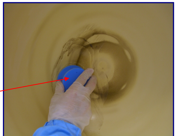
Fig 4: 280 Grit Diamond ScrubPAD scrubbing ceramic dome
