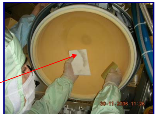
Fig 6: UltraSOLV ® Sponge wiping area free of deposition
