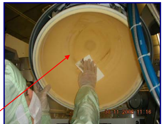
Fig 2: UltraSOLV ® Sponge performing initial wipe of ceramic dome
