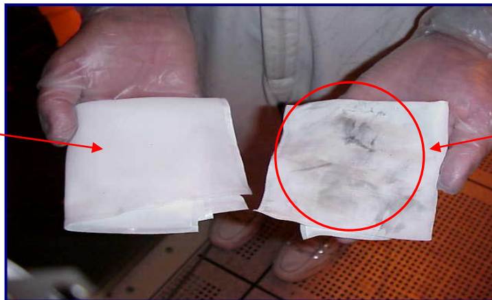
Fig 10b: Particles picked up using HT5790S MiraWIPES ® after completely wiping with current fab wiper
