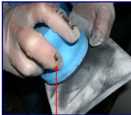
Fig 2: Pull & twist ScrubDISK ® across UltraSOLV ® Sponge
