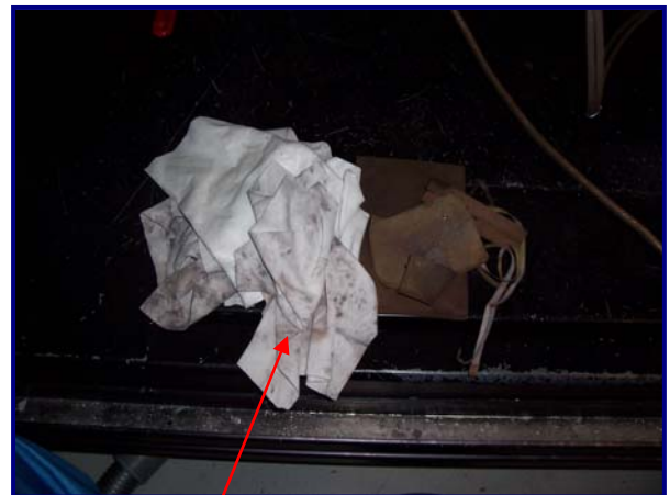
Fig 20: Total amount of hazardous waste generated using Foamtec Vacuum Chamber PM Technique
