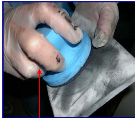
Fig 2: Pull & twist ScrubDISK® across UltraSOLV® Sponge
