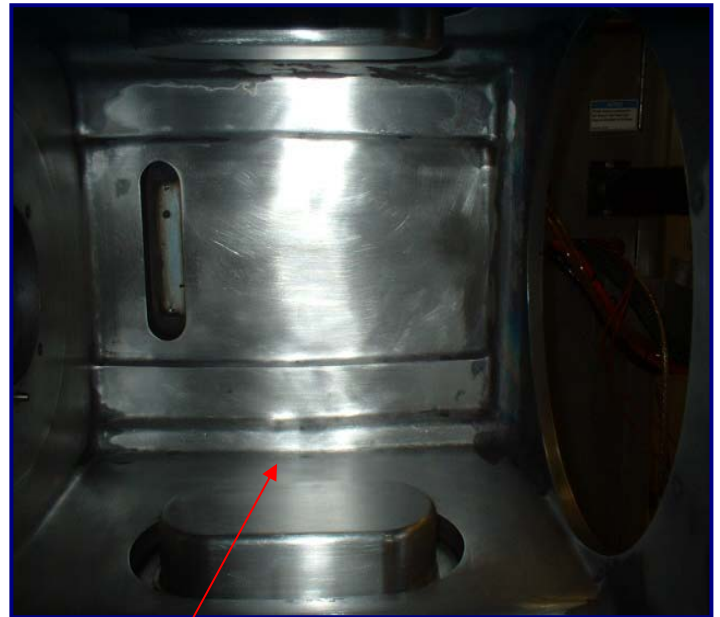
Fig 10 & 11: PM completed using only DI water and IPA for final wipe-down NO H 2 O 2 (Hydrogen Peroxide)
