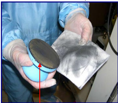
Fig 4: ScrubDISK ® loaded with deposition
