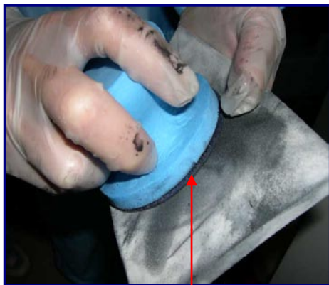
Fig 5: Pull & twist ScrubDISK ® across UltraSOLV ® Sponge
