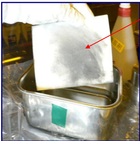
Fig 7: UltraSOLV ® Sponge loaded with deposition
