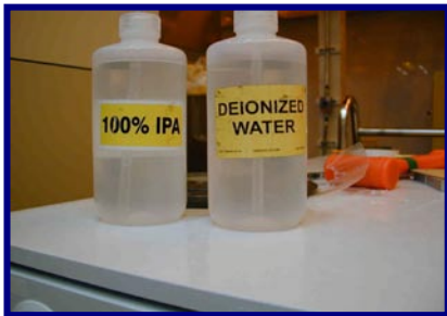
Fig 19: Began PM with both bottles filled. Approximately 30ml IPA and 50ml DI water consumed during PM
