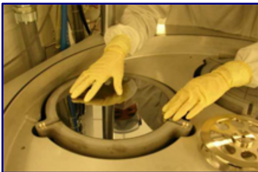
Fig 11: Use dummy wafer to check the backside pressure under spec (<10Torr)
