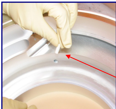
Fig 4 & 5: Placing HT6635B-1 Foam Plug in channel
