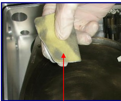
Fig 9: ScrubPAD Loaded with Deposition
