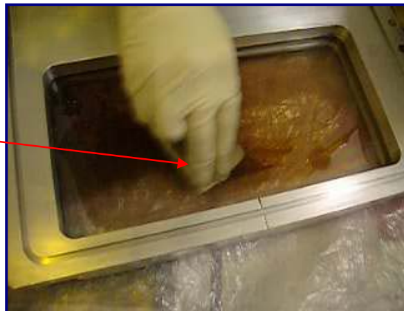
Fig 23: 1350 Grit Diamond ScrubPAD gently removing deposition from window
