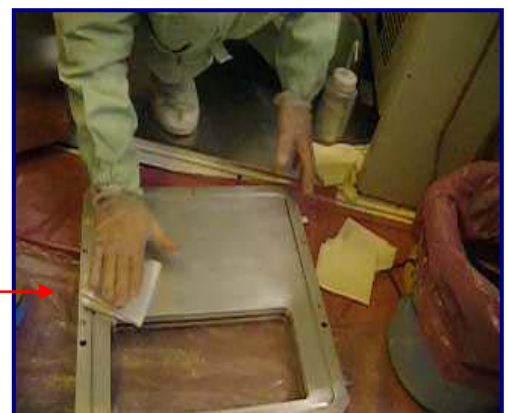
Fig 27: Performing an initial wipe of chamber door
