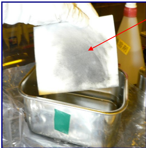
Fig 16: UltraSOLV® Sponge loaded with deposition
