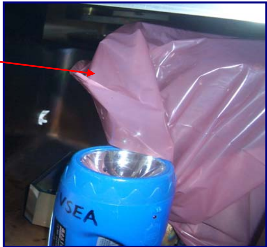
Fig 33 & 34: Electrostatic clamp carefully covered with large plastic bag
