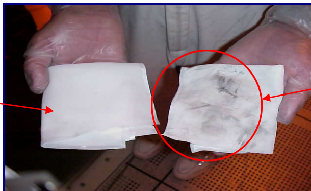
Fig 39b: Particles picked up using HT5790S MiraWIPES® after completely wiping with current fab wiper
