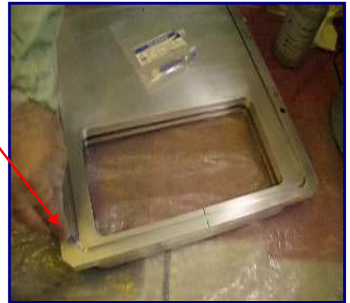
Fig 29 & 30: MiraSWABS ® cleaning out tight areas and grooves along Process Chamber Door
