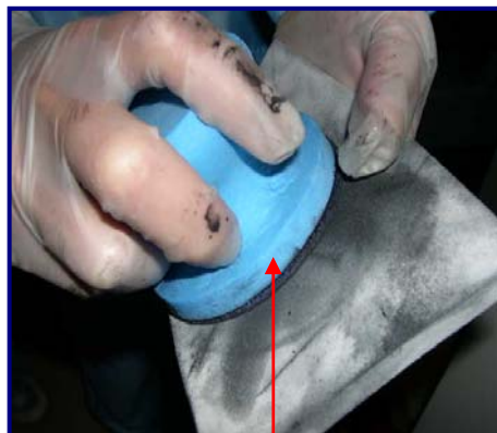
Fig 11: Pull & twist ScrubDISK ® across UltraSOLV ® Sponge
