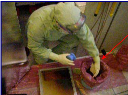
Fig 3: Lightly moisten UltraSOLV® with DI water
