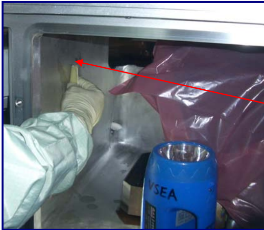
Fig 38: 800 Grit Diamond ScrubPAD polishing process chamber
