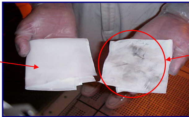
Fig 25b: Particles picked up using HT5790S MiraWIPES® after completely wiping with current fab wiper
