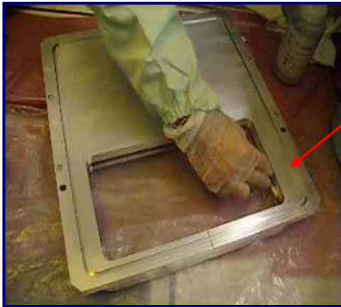
Fig 29 & 30: MiraSWABS ® cleaning out tight areas and grooves along Process Chamber Door
